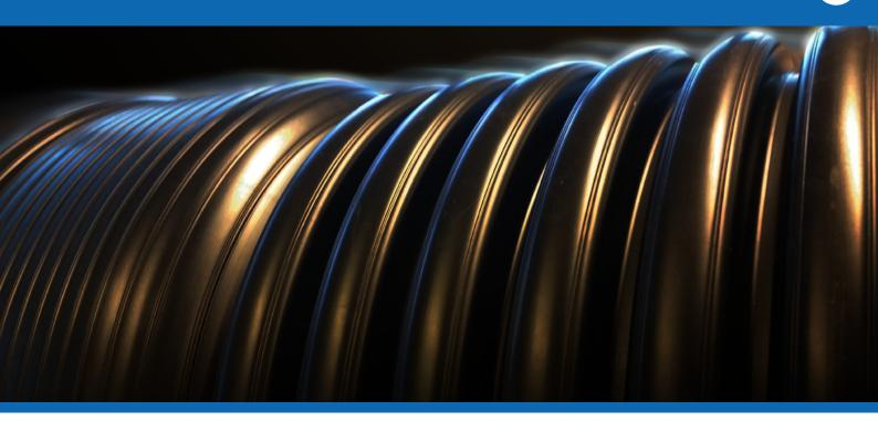
Sewage pipes are produced from PP in diameters Ø 200mm, 250mm, 315mm and 400mm, with a ring stiffness of SN8 (PROLAN/KOMO) or SN4 (AGRILAN). The standard length is 6 meter incl. a welded coupler.
