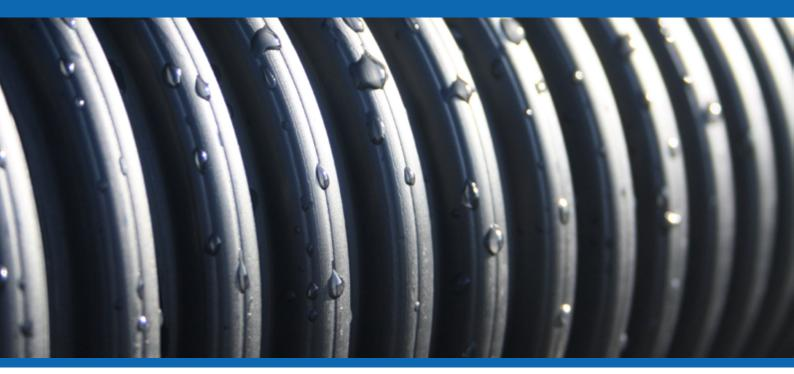
GrainDrain flexible drainage in PE and/or PP is KOMO certified for diameters\* Ø 50mm, 60mm, 65mm, 80mm, 100mm and 125mm. Sizes Ø 160mm and Ø 200mm meet general requirements. GrainPlastics produces both a perforated and an unperforated version.
