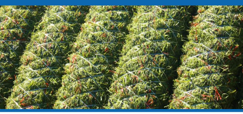
GrainDrain flexible drainage with wrapping GrainFlex1000 (artificial grass-fiber, KOMO certified).
