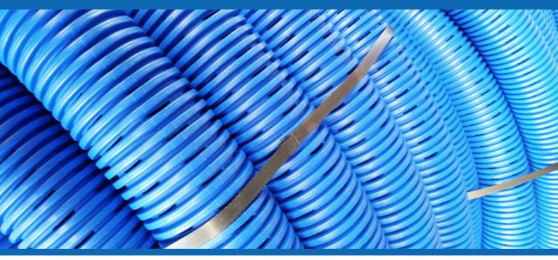
GrainDrain TwinTube flexible double wall drainage in PE is available in diameters Ø 90mm, 100mm, 110mm, 125mm, 160mm en 200mm. TwinTube consists of an outside corrugated pipe with an innerwall on coils or lengths. The advantage in comparison to single wall drainage is a higher ringstiffness and improved waterflow because of the extra innerwall.
