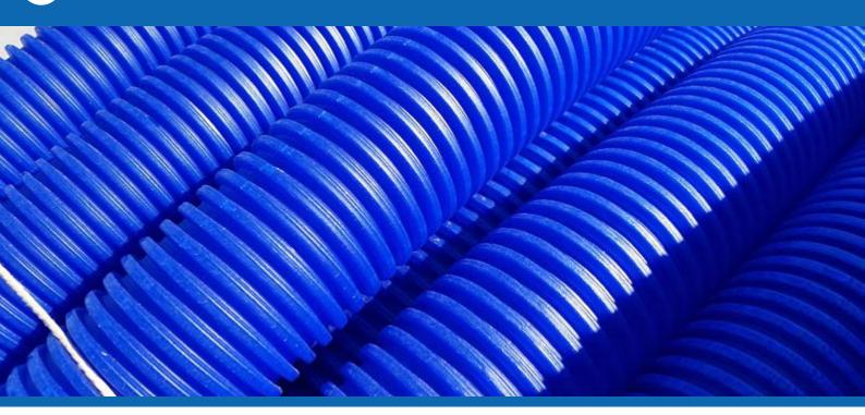
PP suction-tube (Blue), Ø 80 and 100mm, has been developed to withstand forces that are released during usage in combination with pumps. With a ring stiffness of nominal SN10 (ascertained SN14 to SN19) PP blue suction-tube is highly suitable for this heavy job.
